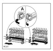
When the top basket is in the higher position it will only take plates up to 20 cm in diameter and you will not be able to use the cup racks.
